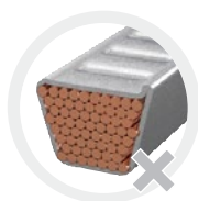
Asymmetrical crimping shape Burr formation on one side
