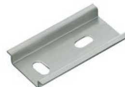
TS 35/7.5 mm according to EN 60715 (s = 1.0 mm)
