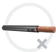
Damaged conductor insulation
